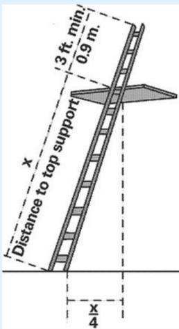
Only use a ladder on stable ground. The footpads should be evenly supported, secured, and level. Stay at least ten feet away from power lines.
